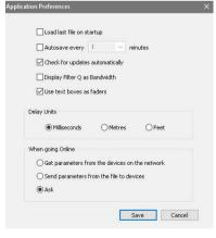
Load Last File on Startup...: Checking this option will cause D-Net to automatically load the last D-Net (\*.NST) that was used, when the application is opened.
