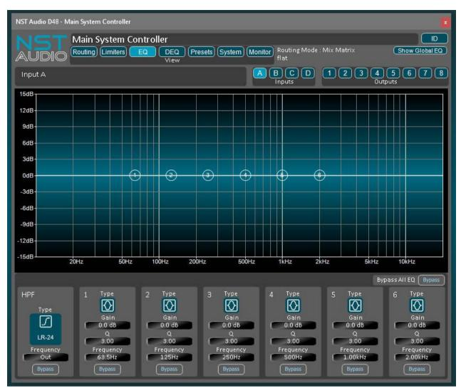
Clicking / tapping on the EQ buttons gives access to all the input EQ parameters. Use the input, A, B, C, D access buttons to edit the desired channel's EQ.
