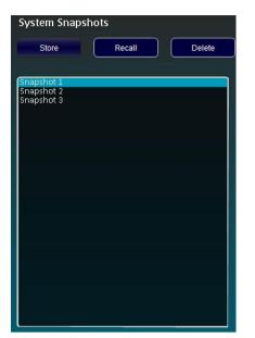
System Snapshots store all of the current settings on all devices defined to memory within the current D-Net (\*.NST) file. This allows quick storing and recalling of settings across the entire current system.
