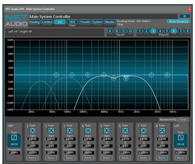
Clicking / tapping on the EQ buttons gives access to all the output EQ parameters. Use the output 1, 2, 3, 4, 5, 6, 7, 8 access buttons to edit the desired channel's EQ.
