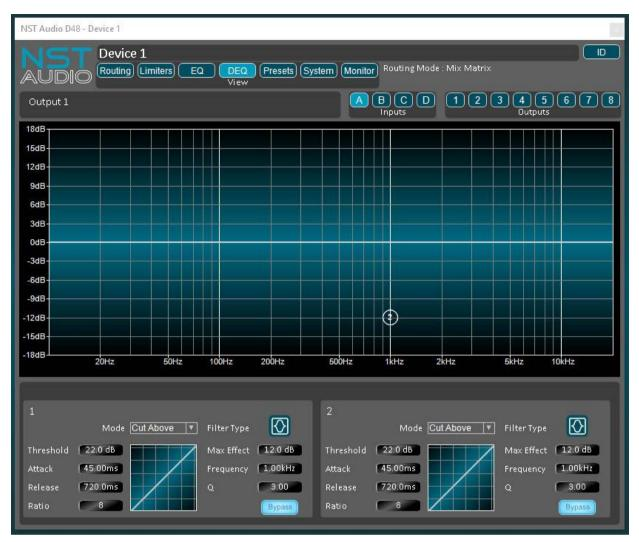
Clicking / tapping on the DEQ button gives access to all the input and output DEQ parameters. \*Note: Dynamic EQ filters are only available when the unit is in 48khz sampling mode (see System Page).
