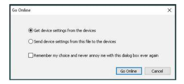
If D-Net finds a matching device, it will ask whether to send the settings to the device, and also give options for identifying the device:
