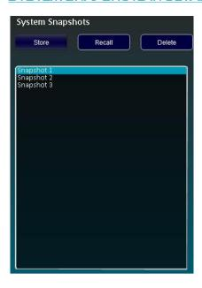
System Snapshots store all of the current settings on all devices defined to memory within the current D-Net (\*.NST) file. This allows quick storing and recalling of settings across the entire current system.
