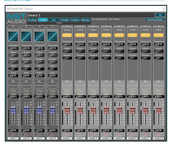
Clicking on the limiter button will show the output limiters instead of the routing.
