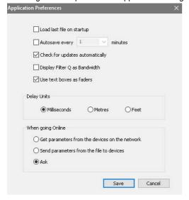
Load Last File on Startup...: Checking this option will cause D-Net to automatically load the last D-Net (\*.NST) that was used, when the application is opened.
