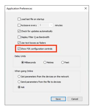
Once this is enabled, the output EQ sections will show the "FIR Config" button:
