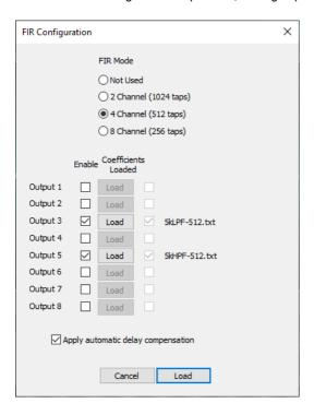
The D48S and ID48S have a total of 2048 FIR filtering taps available at 96kHz. These are available in 3 different configurations :
