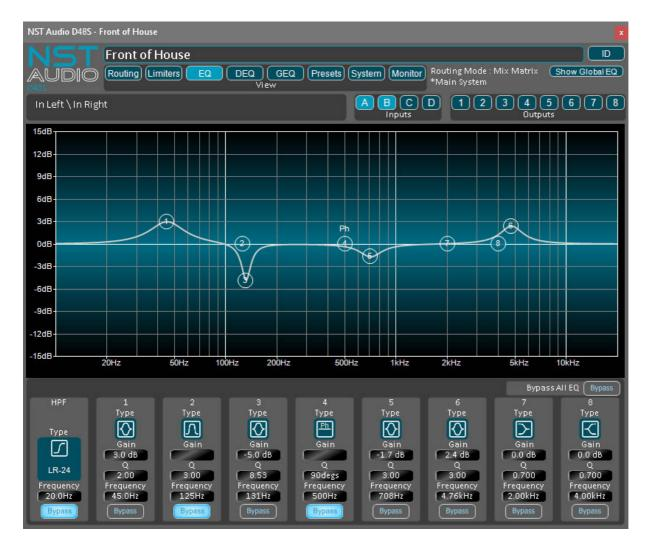
Clicking / tapping on the EQ buttons gives access to all the input EQ parameters.
