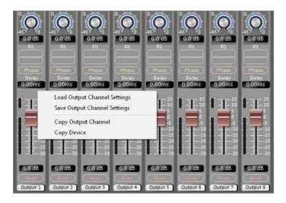
To quickly copy channel settings, or save them to file, right mouse click on an output channel in either the Routing page or Monitor page. Right click another output channel again to paste or load the settings into the channel selected.
