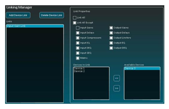
Linking Manager allows various parameter groups to be linked across multiple devices – this allows parameters specified in the link to be adjusted in real time on any device in the link - all devices in the link will respond together immediately to the desired parameter setting.
