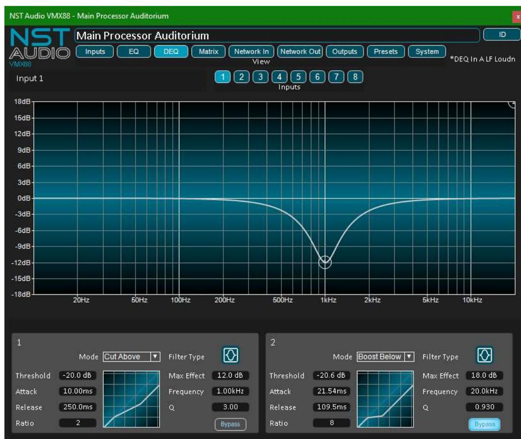
The mini I/O graph in the parameter section shows the Threshold at which gain change will start to happen (the lower knee), and the steepness of this is affected by the Ratio. The upper knee point will move with the value of the "Max Effect" setting, showing that audio exceeding the [Threshold + the Max Effect] point cease to adjust the gain further – so the graph returns to a 45 degree line (or 1:1 ratio) once more.
