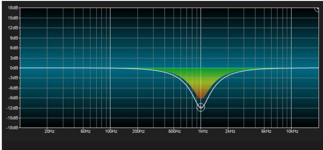
Adjusting the signal level will vary how much the curve fills and the relationship between the “Max Effect” and Threshold controls can be easily seen by turning the incoming audio up and down and observing the effect.
