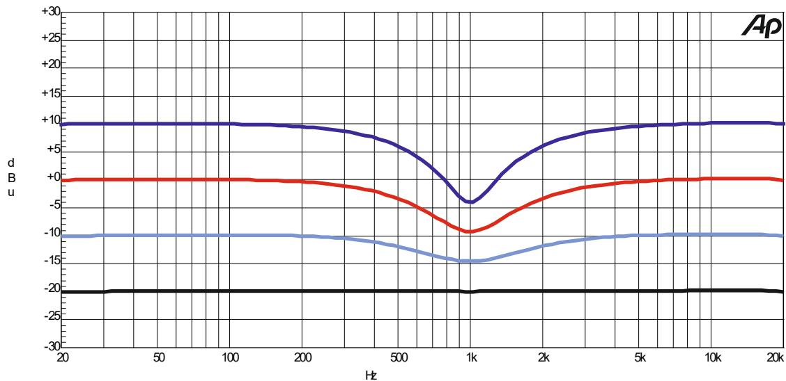
Signals below the threshold will pass unaltered, but as increasing signal is applied, those frequencies centred around 1kHz will be cut or compressed. The ratio in the above example is set at 2:1 so, as with any compressor, the amount of gain reduction applied depends on how much the signal exceeds the threshold. The red line represents a signal at 0dB, which is 20dB above the threshold. At 1kHz, therefore, the signal has been compressed to -10dB or 2:1.
