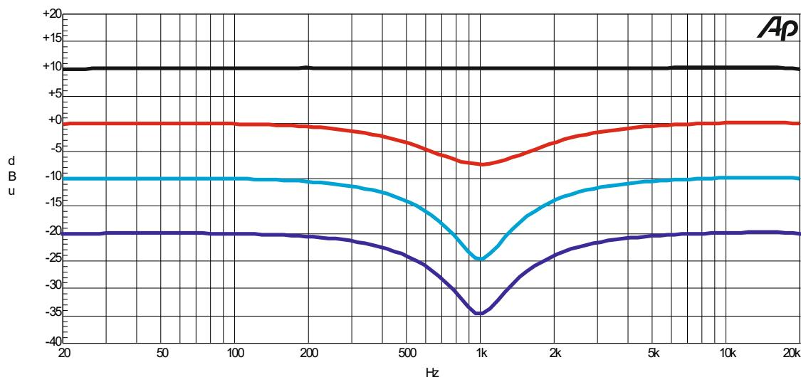
Signals above the threshold will pass flat, but as the level decreases, those frequencies centred around 1kHz will be cut or expanded. The amount of gain reduction applied depends on how much the signal drops the threshold and the ratio set – a 2:1 ratio would mean that for every drop of 1dB below the threshold, the band centred around 1kHz would drop by 2dB.
