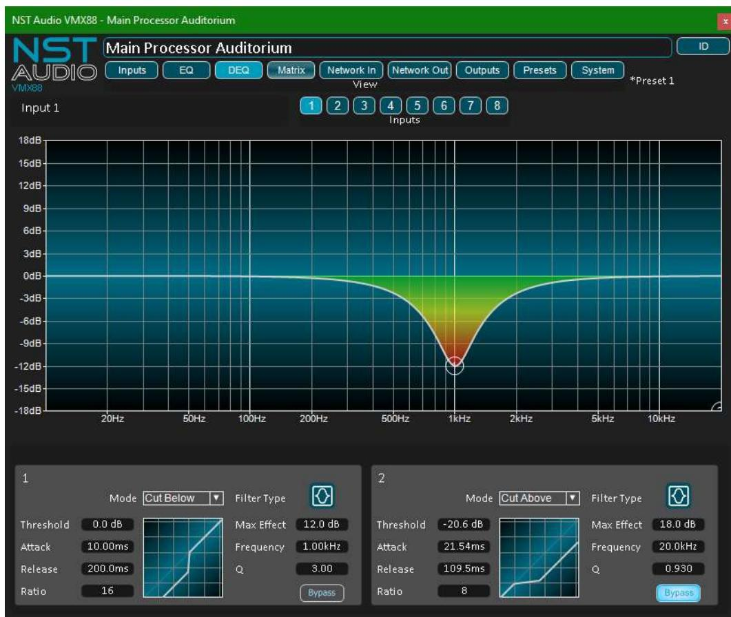
Observing the dynamic effect of audio on the frequency response shows that as the signal level increases, there will be less and less filled in. If the signal stays above the threshold, the curve will simply show the white outline.
