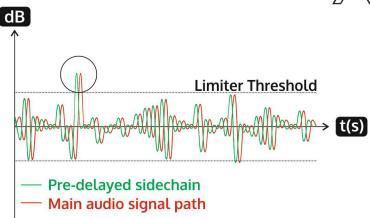
The pre-delayed sidechain is shown in green, with the main signal in red. As the main signal now exists slightly later in time compared to the sidechain, the output from the limiter does not suffer from the overshoot problem. This is because it can begin to react ahead of the main signal's peak and so control it correctly. This is shown in the limiter output below - no overshoot even on the first circled excursion above the threshold.
