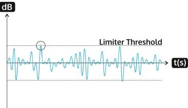
Remember that this delay is only in the order of tens of microseconds, and is a pre-delay – the sidechain is moved back in time in relation to the main signal. Inserting a delay into the main signal path of an analogue dynamics processor will achieve similar results, but with the penalty of delaying the main signal by the amount of look ahead delay introduced.
