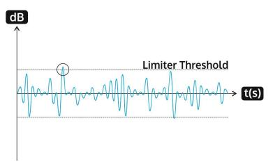
The blue waveform shows the output of the dynamics module. The circled peak demonstrates that the processor has partially "missed" the first peak above the threshold (as it is very fast and short), but has "caught up" shortly afterwards, keeping all other peaks under control. As it is unable to predict what is coming, this will always be a failing with analogue dynamics processing.
