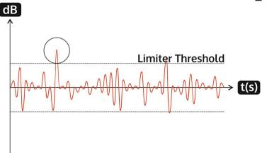
The red waveform represents the input to the dynamics module, with the dotted line showing the threshold for gain control to occur. Peaks above the threshold should trigger a response from the limiter, and so the dynamics processing should react to these as appropriate. (In this case reduce the gain).
