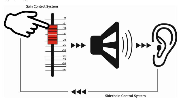
The main signal path is fed through the monitor desk and the gain controlled by adjusting the fader. The sidechain is formed by the feedback path between the engineer's ears checking the level and his brain instructing his hand to turn the fader down if the volume goes over the threshold he has chosen.
