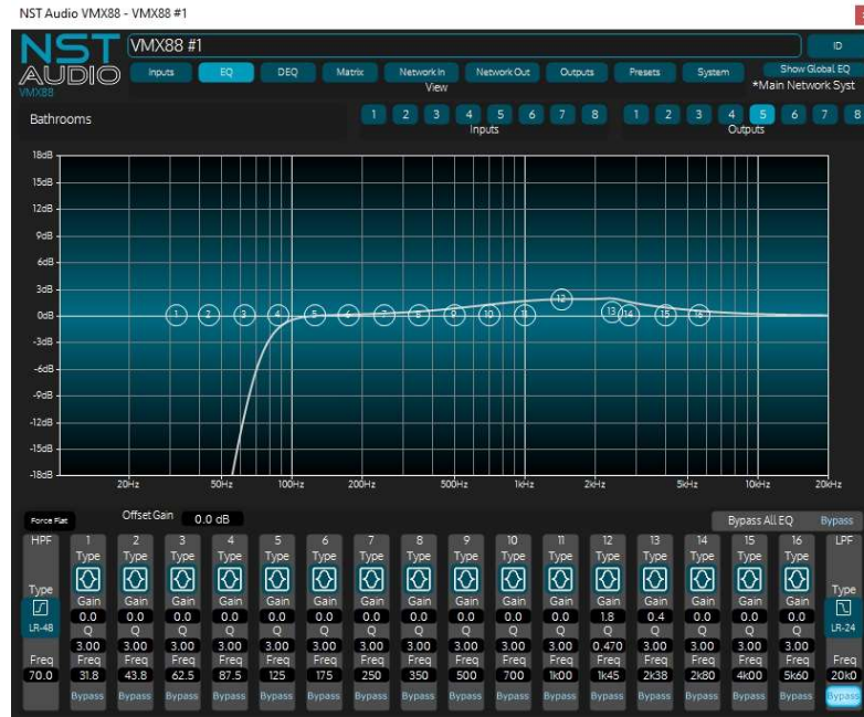
“Bathrooms” zone showing EQ in place.
