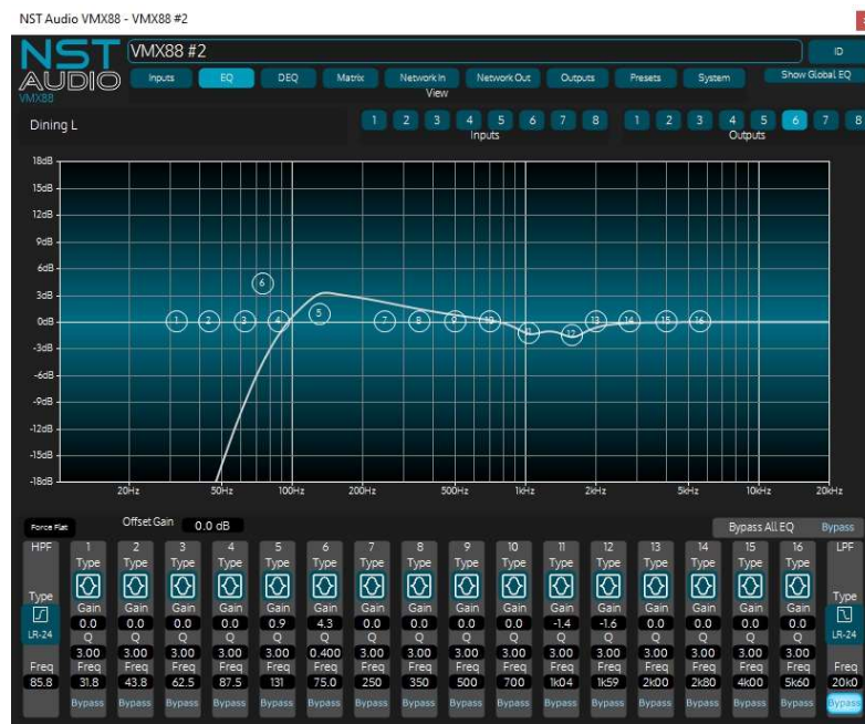
“Dining Room” zone top boxes with light mid EQ cut and roll-off for sub.
