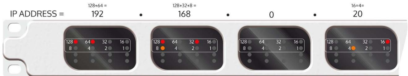
Each window displays that octet's value in binary using the LEDs encoded as outlined above. For example, in the left-most window, the "128" and "64" LEDs are illuminated, so we add these together and that gives 192. In this way, the entire IP address can be decoded.
