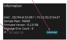
The "Advanced" button then reveals the DHCP status of the device and shows the current subnet mask.
