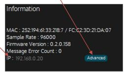
The "Advanced" button then reveals the DHCP status of the device and shows the current subnet mask.
