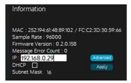
Set the required IP address and press ENTER. Make sure you then press "Apply" to reconfigure the IP address. The device will go offline for a brief period while the network interface resets to use this new address. This will only be for about 1-2 seconds.
