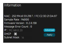
Access the device's IP address settings on the System tab, and press the "Advanced" button. Either set a static IP address in the correct range, or reselect DHCP.
