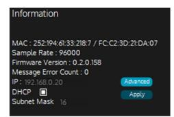
The subnet mask number format is shown in the CIDR format, where the shorthand mask value is appended onto the end of the IP address. This is normally shown in the form 192.168.0.20/16 with the /16 being the subnet mask. It is separated it out in D-Net allowing it to be hidden unless required.
