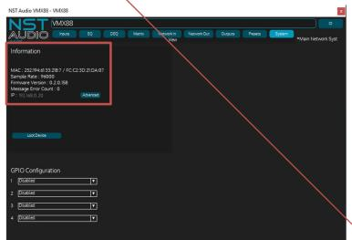
In this instance the device's IP address is set to 192.168.0.20.
