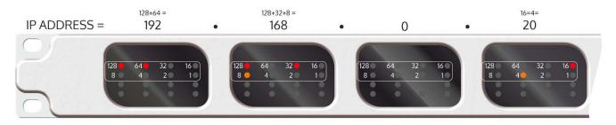
Each window displays that octet's value in binary using the LEDs encoded as outlined above. For example, in the left-most window, the "128" and "64" LEDs are illuminated, so we add these together and that gives 192. In this way, the entire IP address can be decoded.
