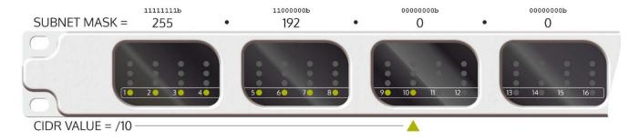
The subnet mask display uses a different technique in keeping with the CIDR notation used to show it in D-Net. The bottom row of meter LEDs (green) show an increasing number from left to right, directly representing the subnet CIDR format value. In this example, 1-10 are illuminated so the subnet mask is set to 10 which equates to 255.192.0.0 if we refer back to the table on page 14.
