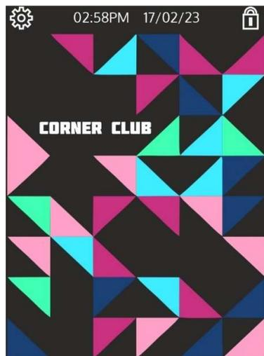
**Set Screensaver:** The NST Logo shown when the VR2 displays the screensaver can be changed to match the venue's. The required file format is 24-bit RGB, in png format, with a max resolution of 320W x 320H pixels.
