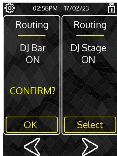
On the VR2, routing screens work virtually the same as preset recalls, except that after the confirmation query, the screen doesn't show an "ACTIVE" message.
