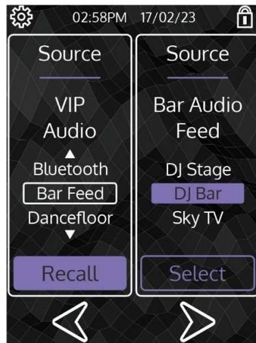
On the VR2, pressing “Select” enables the rotary to scroll through the sources that have been defined and pressing “Recall” will then switch the sources and highlight the choice.
