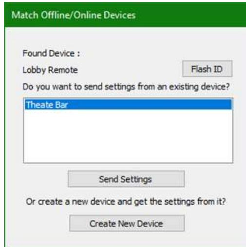
Press the Flash ID button to check which live VR2 is going to receive the settings. It will flash the NST logo and bezel in blue for five seconds. This is useful if there are multiple VR2s on the system.
