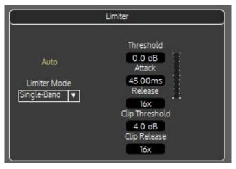
There are two more parameters normally associated with setting a limiter. These are the Attack and Release times.
