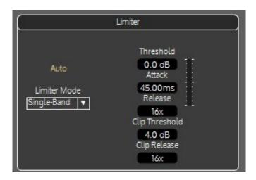
Limiters help prevent the audio level from either getting so high that it will damage the speakers.
